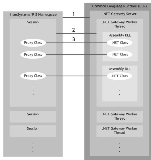
Instances of the .NET Object Gateway Server run in the CLR. InterSystems IRIS and the CLR may be running on the same machine or on different machines. The numbered items in the *.NET Object Gateway Operational Model* diagram point out the following relationships:
