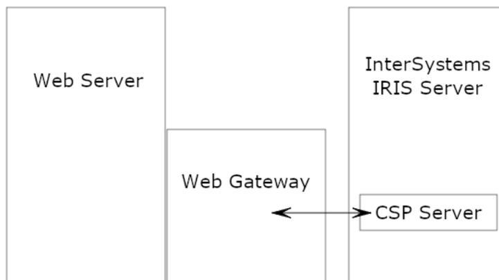
The web server and the CSP server may be implemented by one or many computers. During development, all three components (web server, Web Gateway, and CSP server) may be on a single machine. In a large scale deployment, there may be multiple web servers and CSP servers in two- or three-tier configurations.
