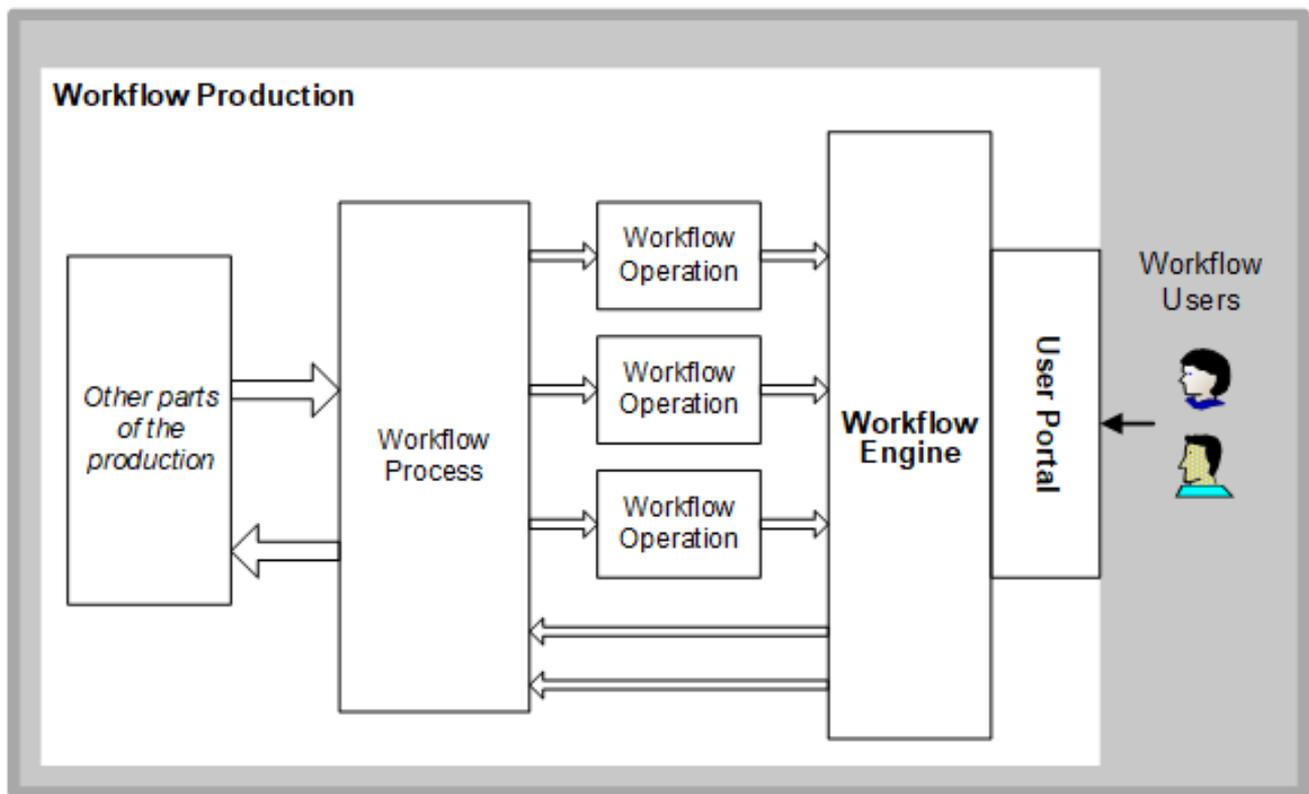
A *workflow process* is a BPL process that sends task requests to workflow operations. This process is responsible for coordinating work among these workflow operations. It might also invoke standard business operations (that is, ones that do not require human intervention). Both types of element may be required to complete the business process.
