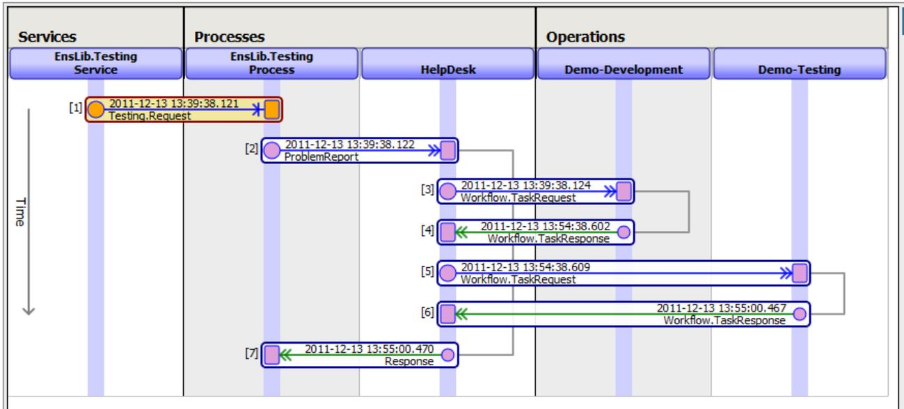
This example shows a session in which a task request was sent to the Demo-Development role and was addressed by a user in that role. Then the workflow process (HelpDesk) sent another task request to the Demo-Testing role. A user in that role addressed the request and the workflow process sent a response to the process EnsLib.Testing.Process.
